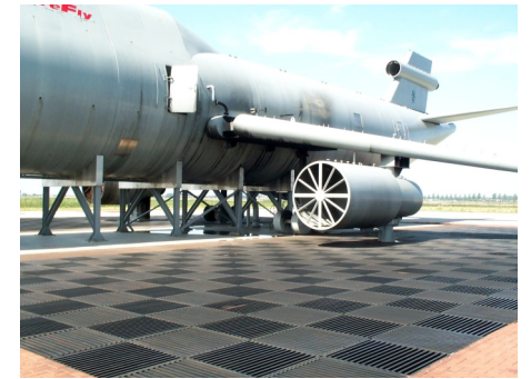
Patented "Drive-On" Fuel Spill allows rescue vehicles to drive right up to the aircraft mockup.
