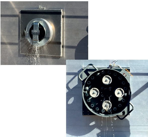
training dome leak simulation
