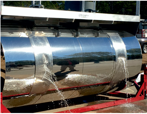
tank fuel leak simulation
