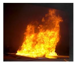
Interior Aviation Flight Deck 15 x 15 Foot Five Zone Fuel Spill Fire
