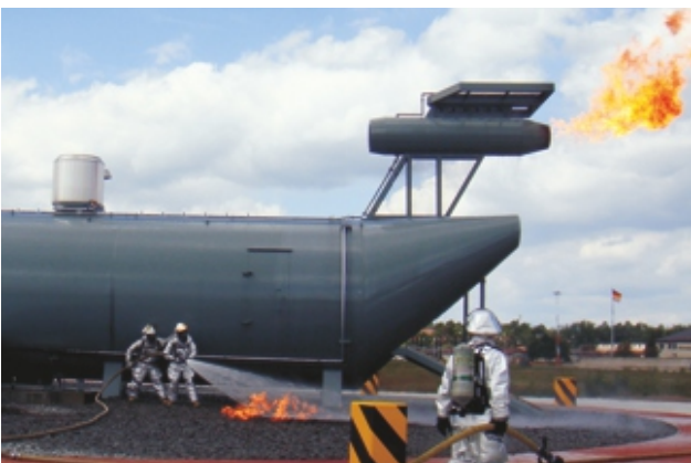
Tail Engine Fire and Fuel Spill
