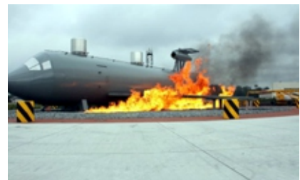
Fuel Spill at Jet Engine Wing
